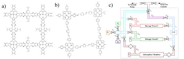
Figure 1. Chemical structures of porous (a) Cobalt phthalocyanine, (b) Cobalt porphyrin (c) Schematic of the proposed volumetric adsorption setup.
